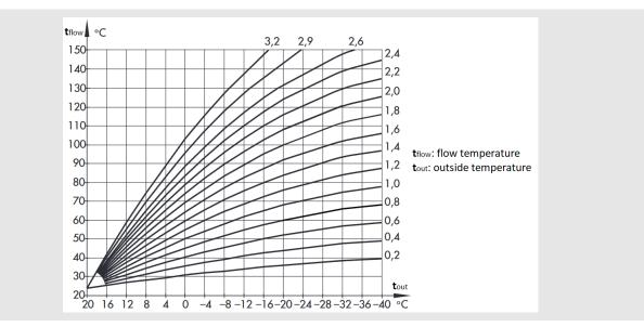
Figure 12: Heating characteristics using the example of TROVIS 5573 [Samson, (2023)] [3]
