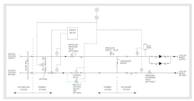
Figure 15: Direct connection of building installation to district cooling system [Skagestad & Mildenstein 2002] [4]
