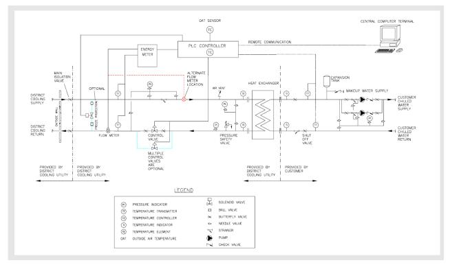
Figure 14: Indirect connection of building installation to district cooling system [Skagestad & Mildenstein 2002] [4]
