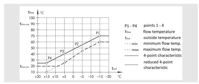
Figure 13: 4-point characteristic usingTROVIS 5573 [Samson, (2023)] [3]
