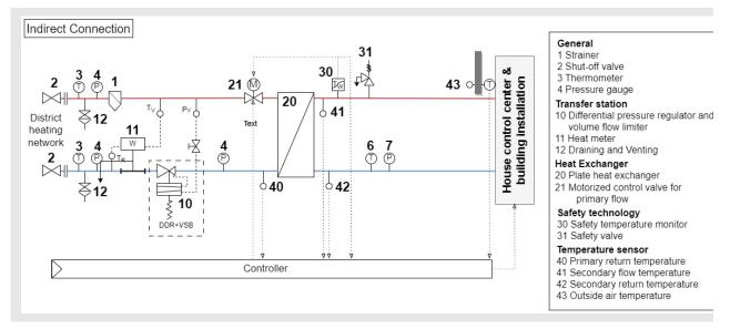
Figure 5: Indirect connection between building installation and thermal grid
