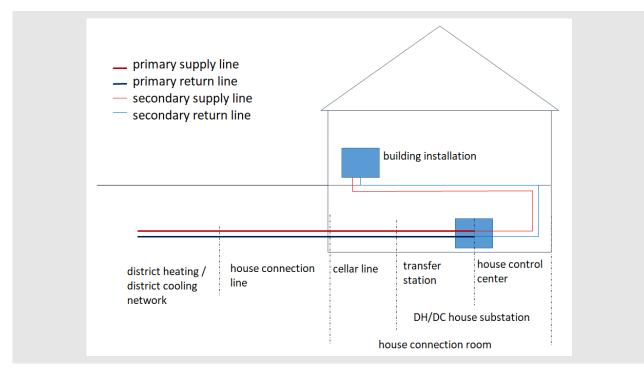
Figure 3: Heat transfer from the district heating/cooling network to the building using house substations
