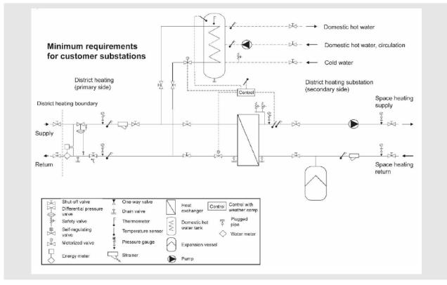
Figure 18: Minimum requirements for customer substations
