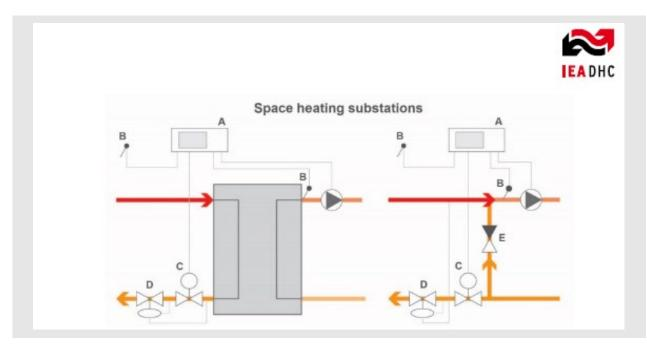
Figure 6: Example of the basic layout for an indirect (left) and a direct (right) space heating substation
