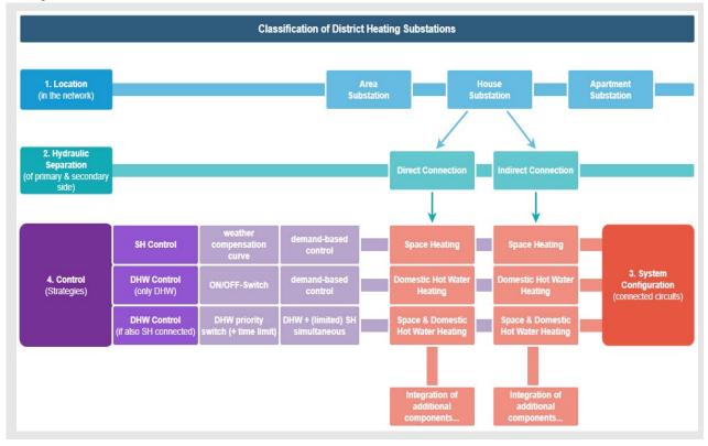
Figure 1: Classification of DH substations
