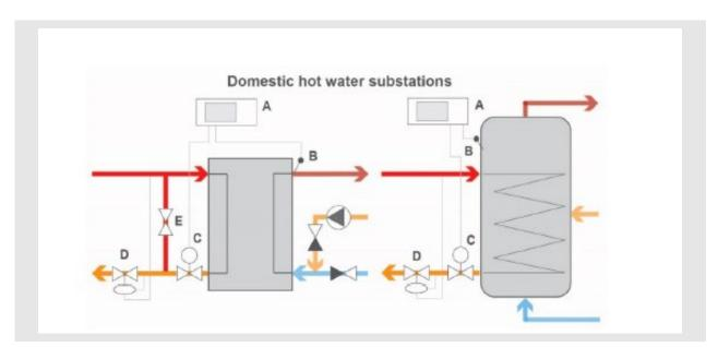
Figure 11: Example layout of a domestic hot water heat exchanger (left) and a domestic hot water storage tank (right)
