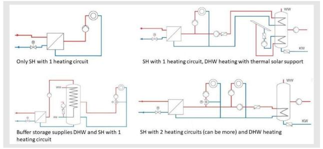
Figure 9: Example of different system configurations connected to the thermal grid
