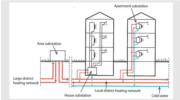
Figure 2: Differences between area, house and apartment substations [Frederiksen, & Werner, (2013)] [1]
