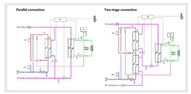
Figure 17: Parallel and two-staged connection
