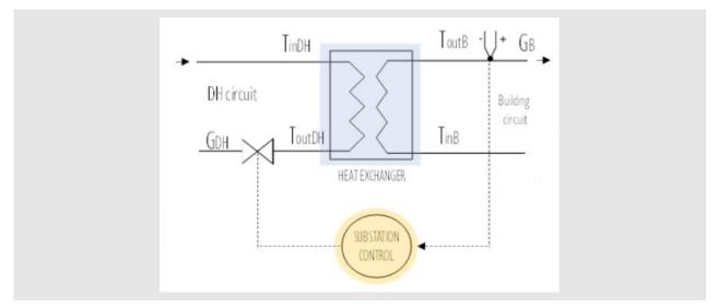
Figure 7: Heat exchanger and notation for key variables
