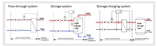
Figure 10: Types of domestic hot water heating systems
