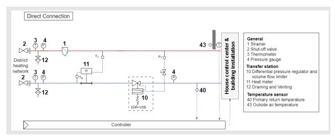
Figure 4: Direct connection between building installation and thermal grid
