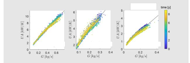
Figure 8: Examples of variation of UA depending on mass flow rate [2]
